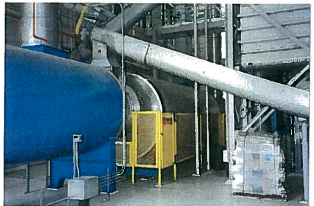
Figure 4. Rotary Dryers, the Most Common Type Used for Drying Wastewater Solids.
