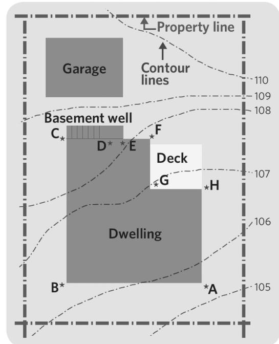
**Example:** to calculate natural grade elevation:
