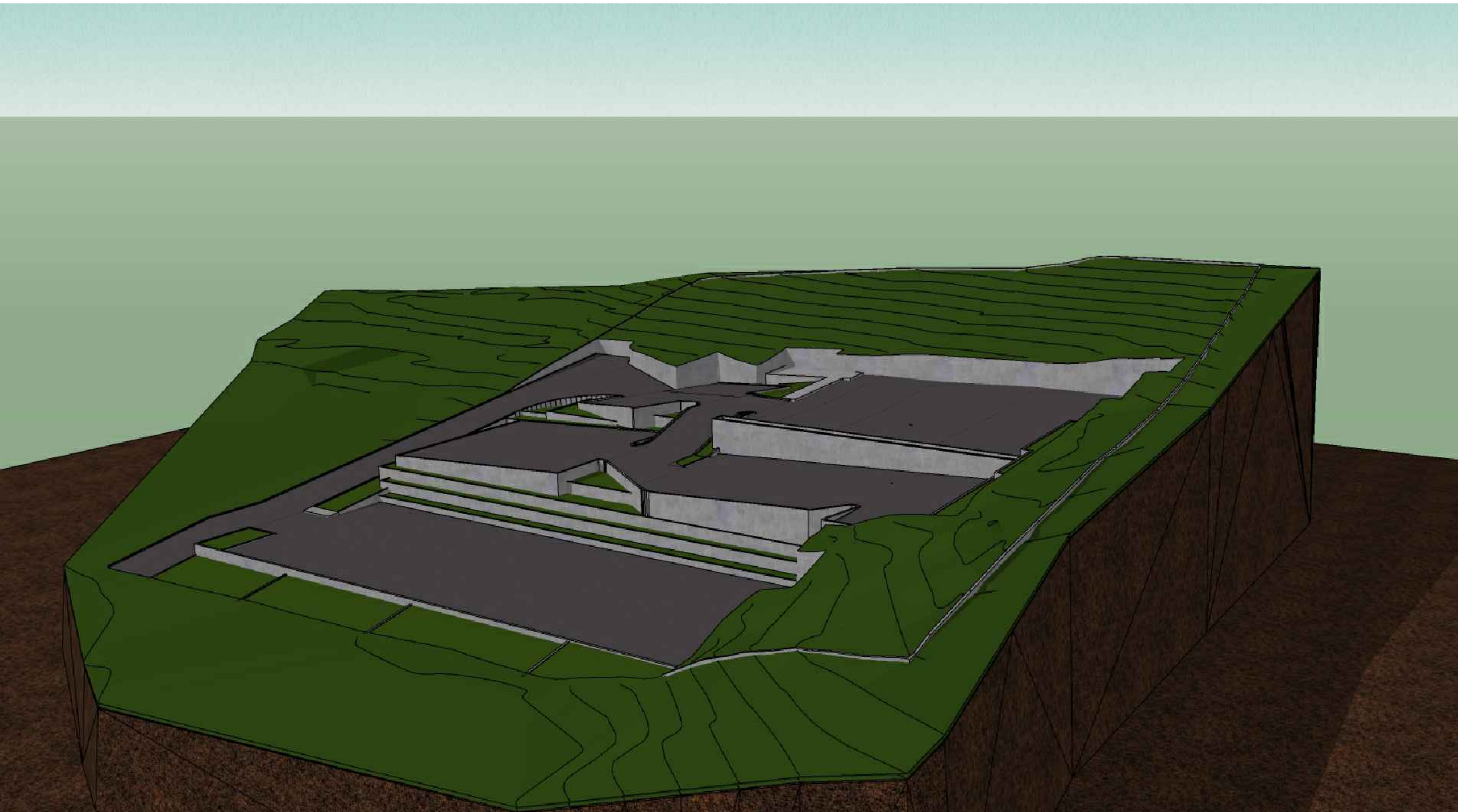
SITE WITH CUT AND FILL
