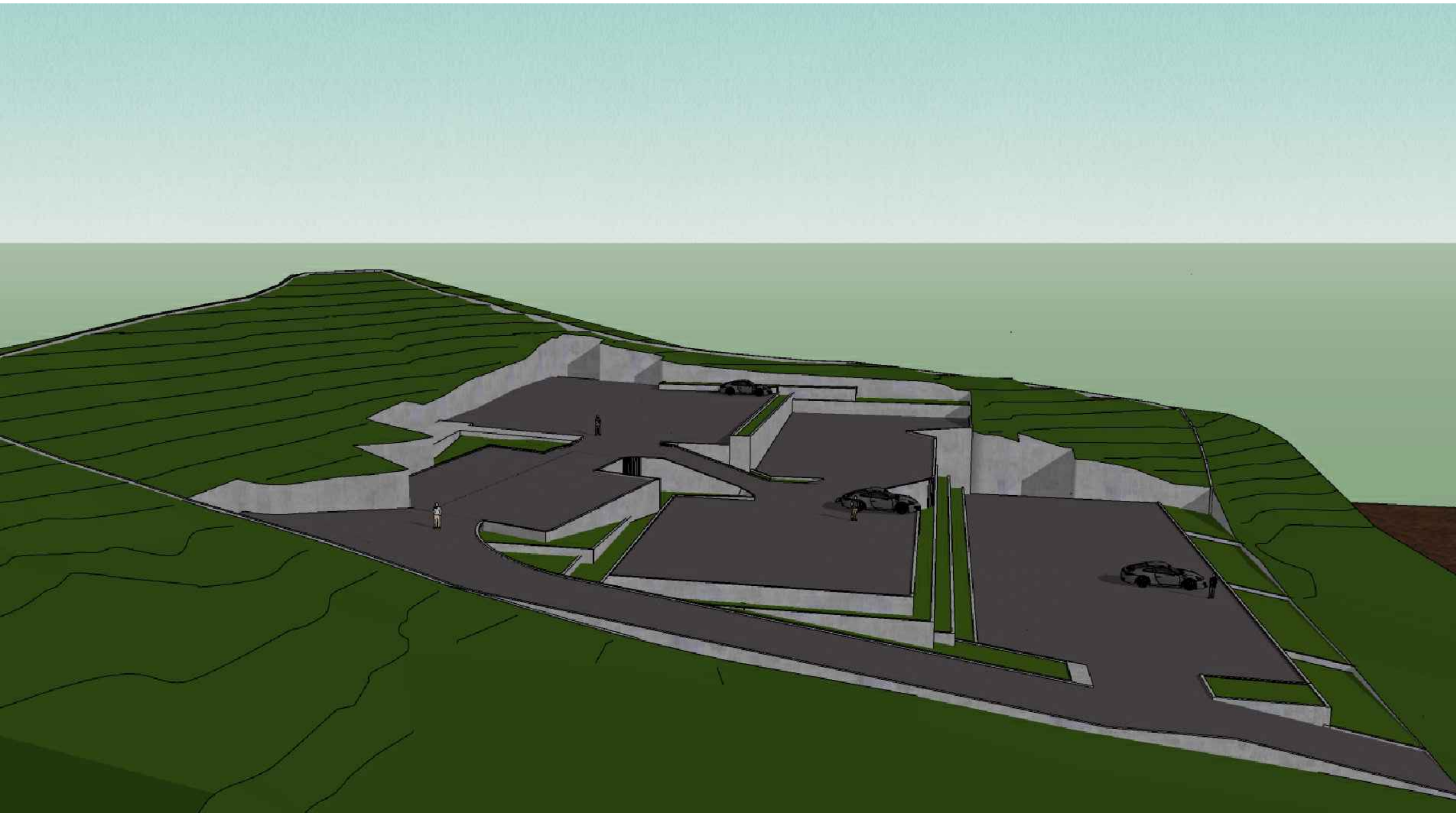
SITE WITH CUT AND FILL
